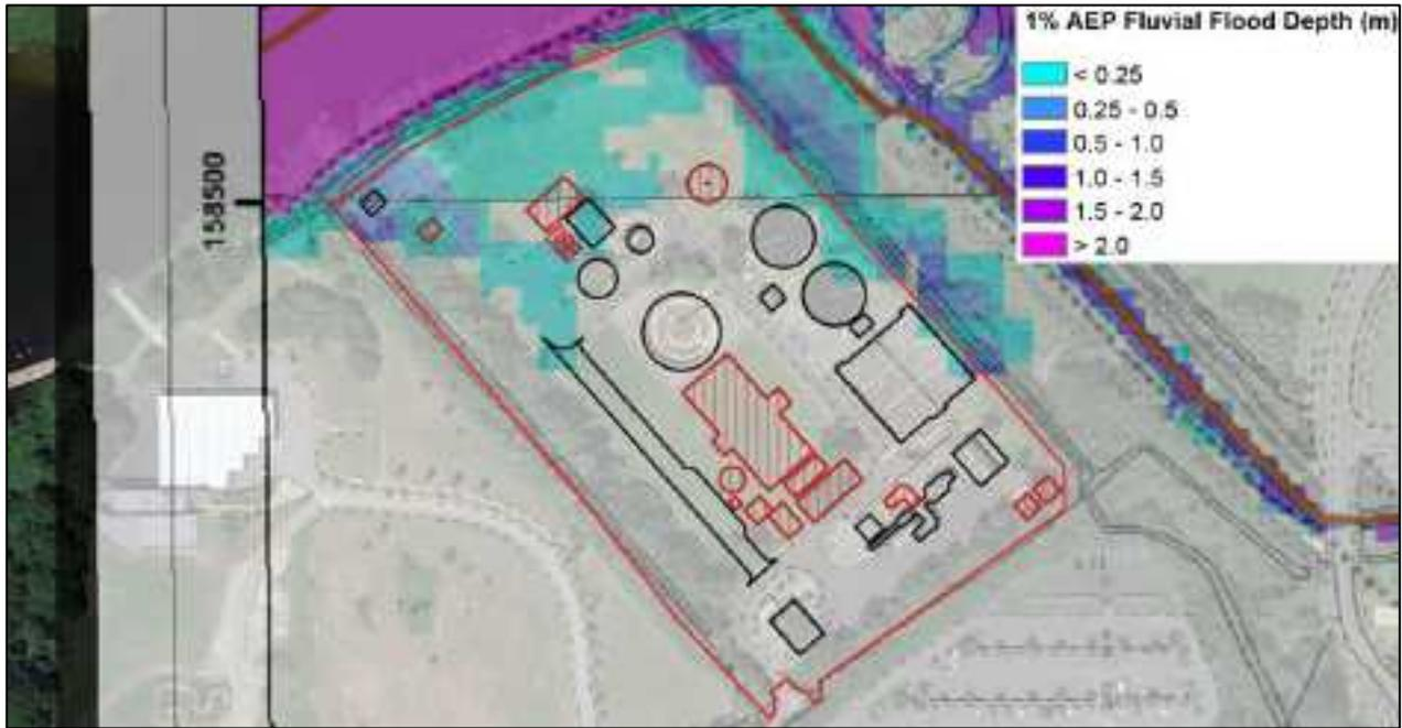
**Figure 15: Flood Depth Map (1% AEP) with proposed infrastructure**
