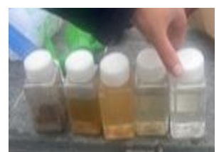
Water samples at various stages in the filter process
