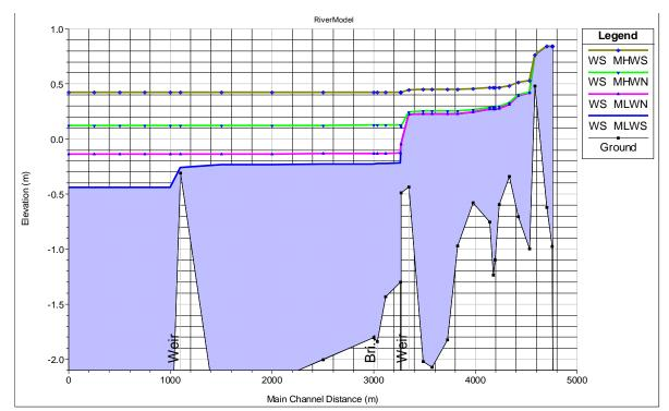
Figure 2.14 - River longitudinal section, modelled water profiles for Q=3.09m<sup>3</sup>/s
