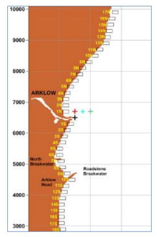
Figure 5.7 - Model sampling strips for effluent concentration estimates
