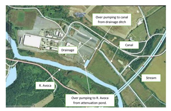
Figure 3.1 Drainage at the IFI Site
