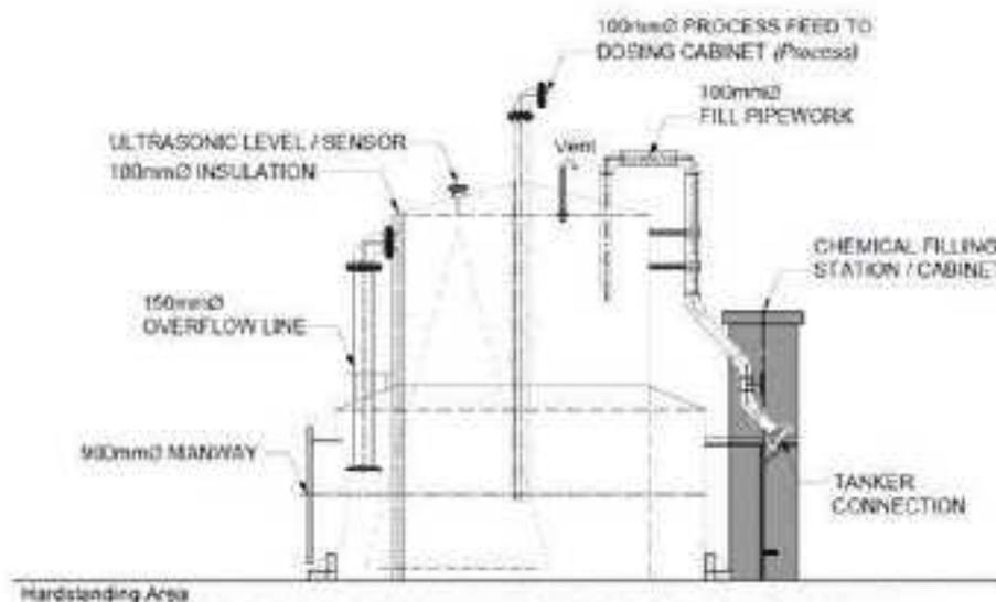
**Figure 3 Sectional view of typical circular free standing chemical storage tank.**
