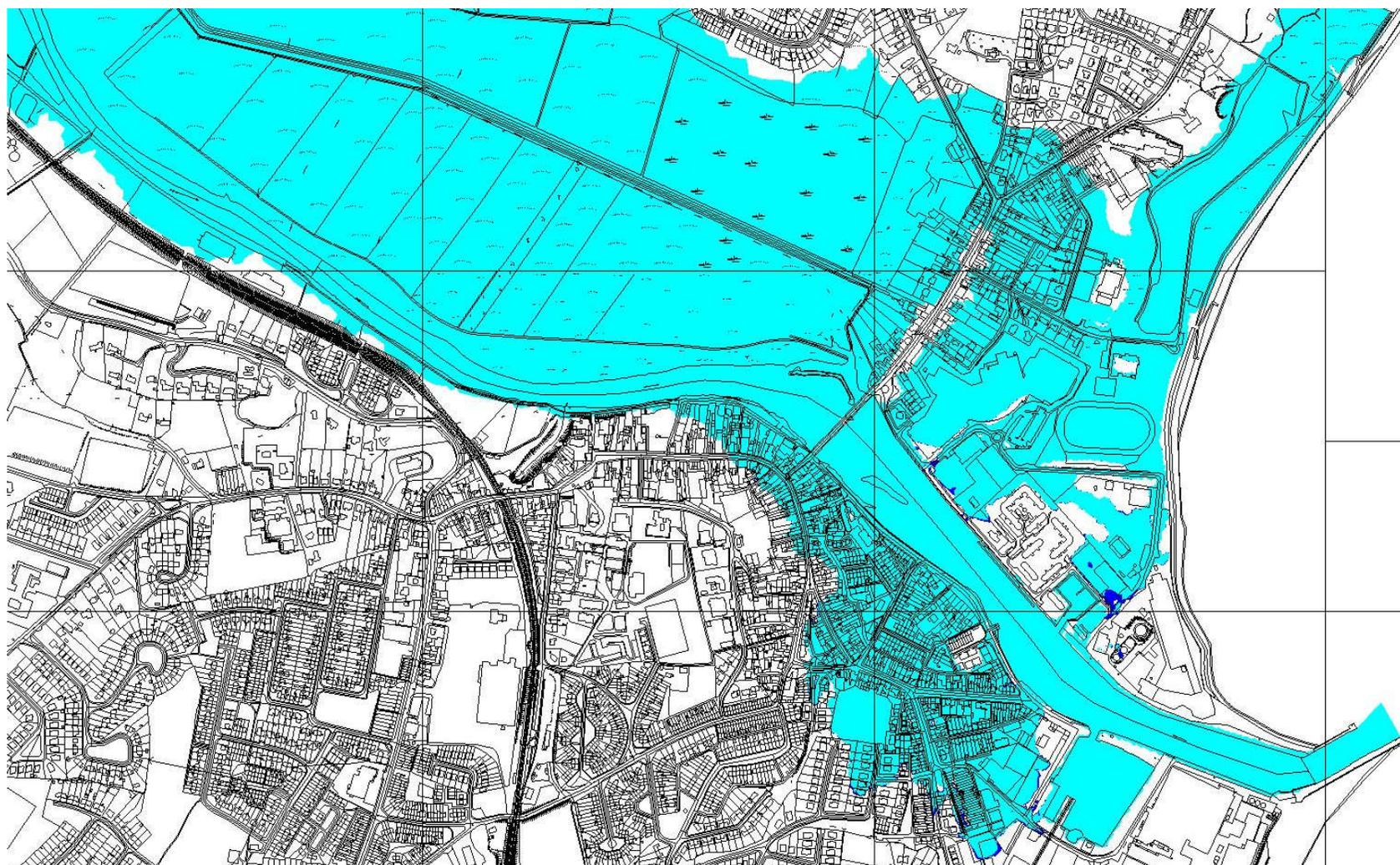
**Figure 16: Predicted Flood Extents for existing and proposed temporary haul road downstream and Bridge arch underpinned and in-channel works completed at the bridge including upstream manhole encroachment. (Blue existing baseline and Cyan proposed construction) (overall minor reduction in the flood extents- very slight beneficial impact)**
