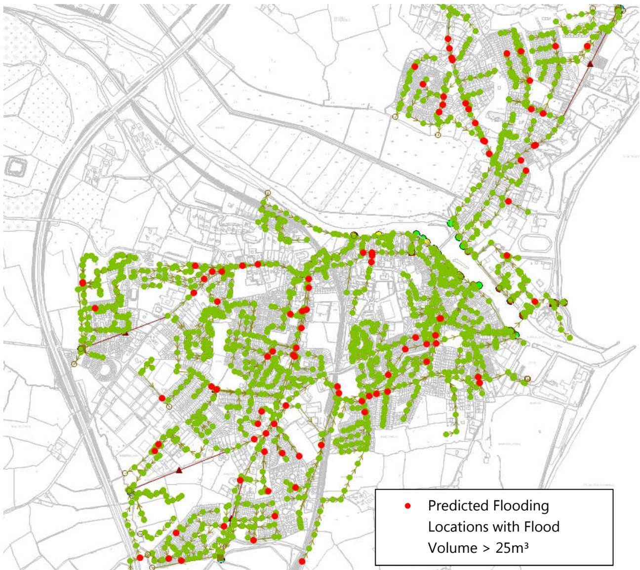
**Figure 2:** Existing System with Interceptor Sewer - Predicted flooding location > 25m<sup>3</sup> for M30\_60 & MHWS with CC
