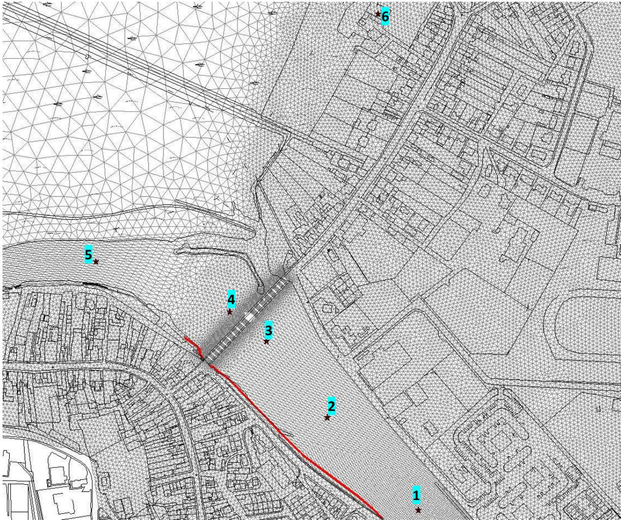
**Figure 4: Reference Site locations within the Avoca River Channel for flood level impact prediction between existing and proposed Interceptor**
