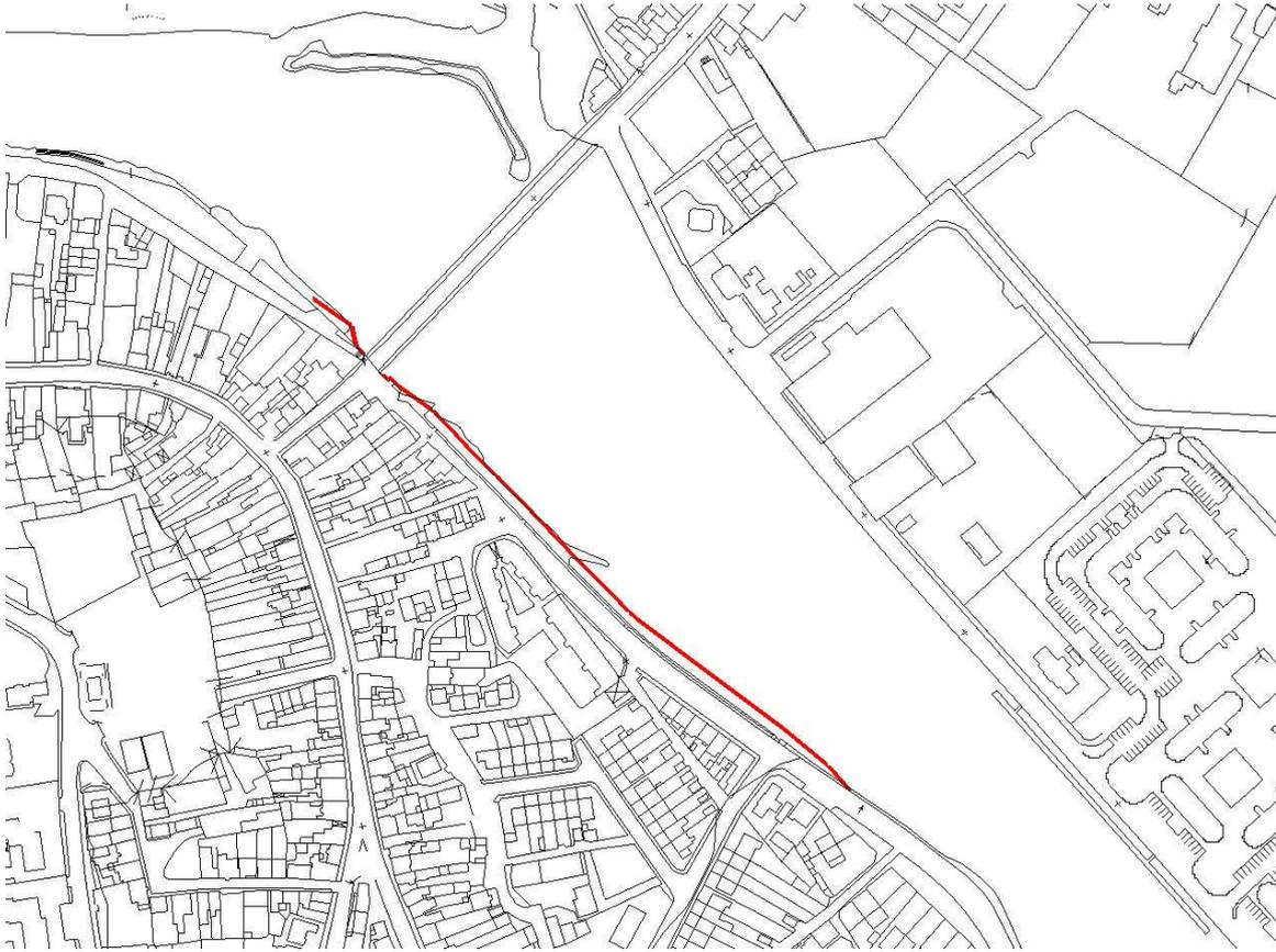
**Figure 1: Proposed encroachment and new position of Quay Wall shown in Red**
