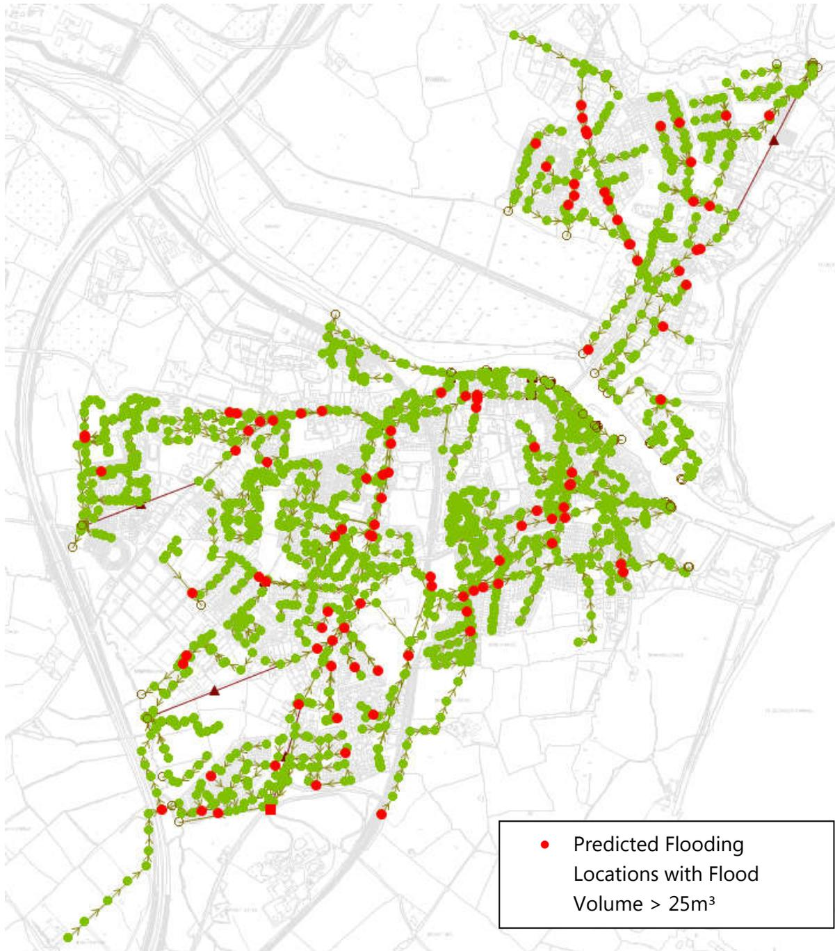
**Figure 2:** Existing System - Predicted flooding location > 25m<sup>3</sup> for M30\_60 & MHWS with CC
