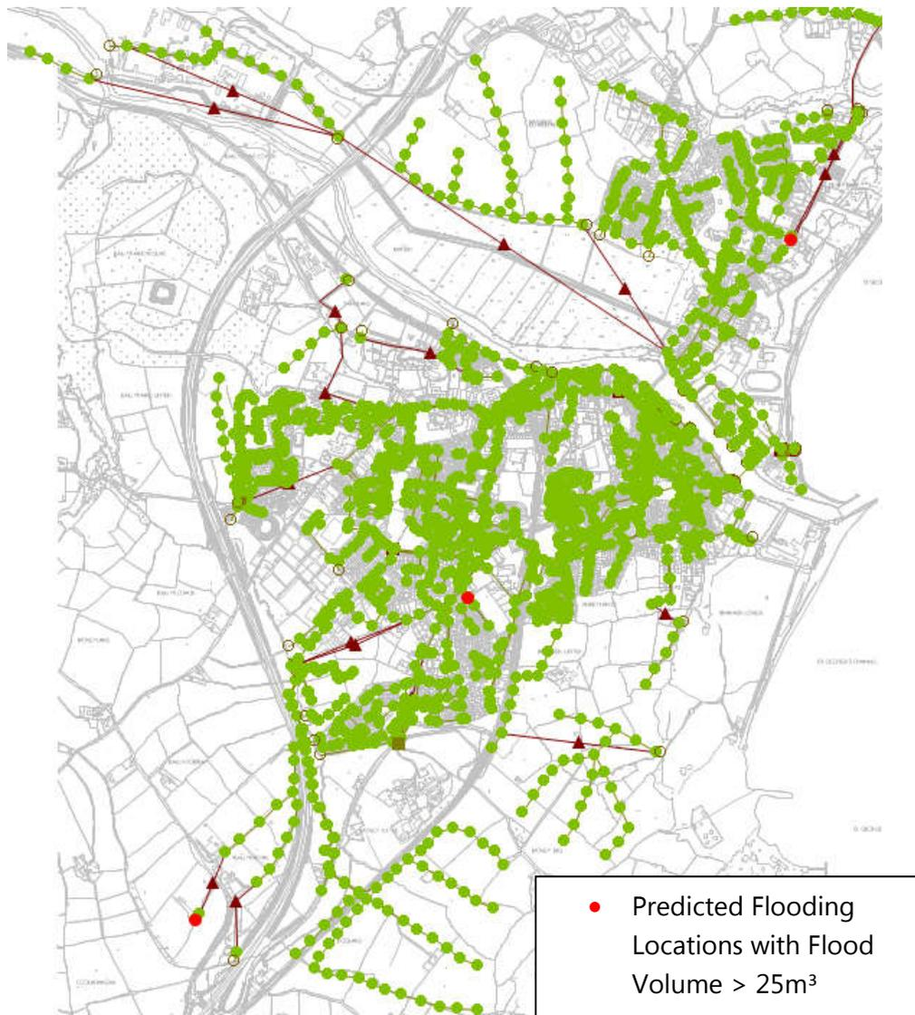
**Figure 3** Scenario 1 - Predicted flooding locations with flood volume > 25 m<sup>3</sup>
